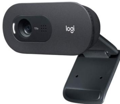
Figure 5 USB webcam used for the vision system.
